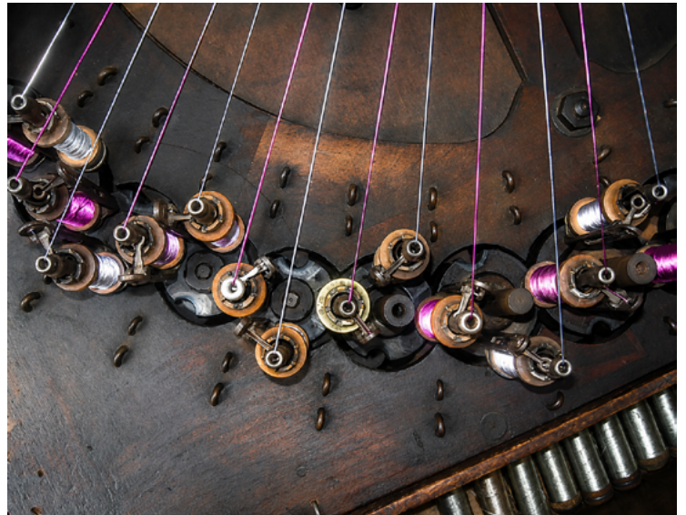
Photograph of spindles in action on a loom, showing threads fanned out and converging toward the braiding point.
